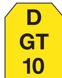
BEGINNING OF GRADE TIMING SECTION IN APPROACH TO "GT" SIGNAL WHEN A DIVERGING ROUTE AHEAD "10" DENOTES MILES PER HOUR
